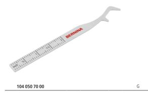
With the CS-Lock Tool, the needle threads can be pulled between foot and stitch plate easily. This eases cutting and locking the cover- and chainstitch. The scale serves as tool to measure hems, seams or mark fabrics. In addition the scale can be used to adjust the seam guide.
