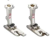
stitch hemmer creates a hem with particularly beautiful stitching. The fabric is folded over twice in a single operation as it is sewn with a straight-stitch. Feet #62 and #64 are used for hems with a width of 2 and 4 mm respectively.
