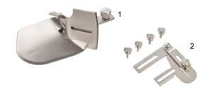
With the single fold binder attachment, fabric edges and necklines can be perfectly bordered with bias tape. The unfolded tape is inserted through the attached guide rail, folded over on the upper side while the under side remains open, and is then sewn on with a cover stitch. For the perfect look, the bias tape can also be self-made.
