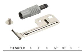
The pintuck attachment facilitates the sewing of corded pintucks. Simply guide the filler cord through the channel of the attachment. When used in conjunction with the pintuck foot, the cord is automatically incorporated in the pintuck, creating a beautiful raised effect.
