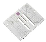
Color-coded purple, this stitch plate has a reduced needle-hole width of 5.5 mm. Suitable for all 9 mm machines, it achieves particularly good results when sewing thin or soft materials. All zigzag and decorative stitches up to a width of 5.5 mm can be used to create detailed sewing projects.
