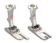
This foot enables precise lap seams to be produced. Since both seam allowances are enclosed and stitched securely in the hem seam, the foot is also suitable for sewing reversible clothing. Foot #70 is suitable for lap seams up to 3 mm wide, whilst foot #71 is suitable for lap seams up to 6 mm in width.
